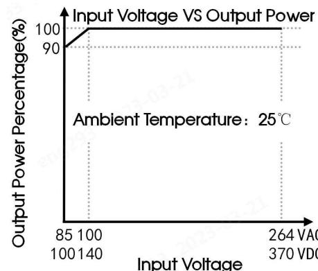
Note: 1. With an AC input voltage between 85-100VAC and a DC input between 100-140VDC the output power must be derated as per the temperature derating curves;
